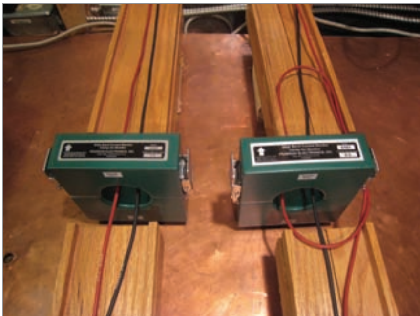
Figure 10: CM measurement on left; dm measurement on right.
