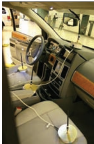
Figure 5: Example of on-board transmitter testing
