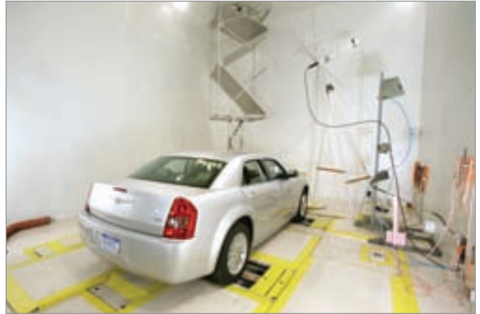
Figure 4: Example of a vehicle in a reverb chamber
