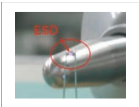
Figure 6: ESD air-discharge to 0603 MLCC
