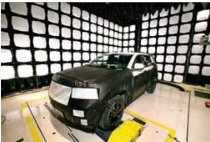
Figure 6: Vehicle in an anechoic chamber for RF emissions testing
