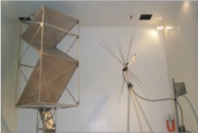
Figure 3: Typical paddle/stirrer (left) in a reverb chamber and two radiating antennae (right)
