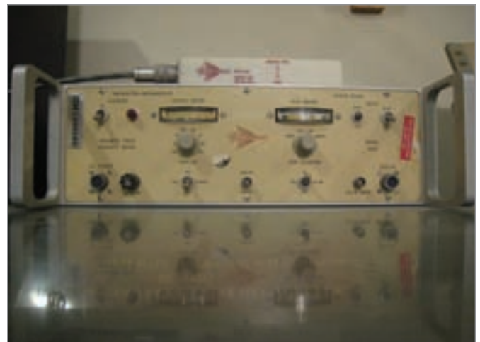
Figure 1: Electro-Mechanics Company EMCO 6640 variable- \mu magnetometer (circa 1964).
