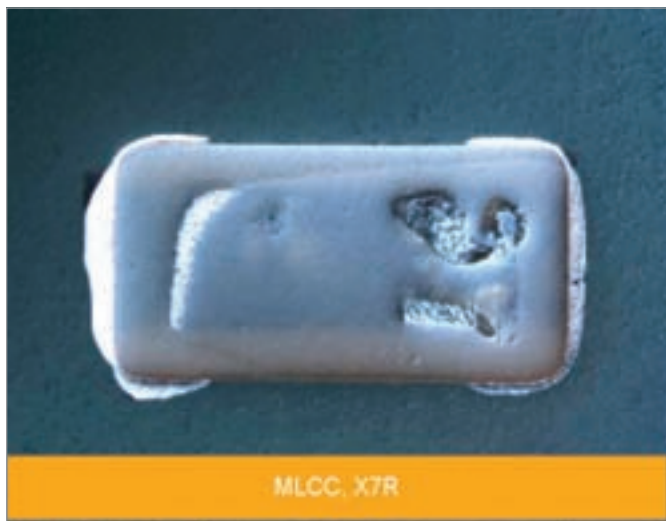
Figure 10: Dielectric damage for post-ESD X7R MLCC
