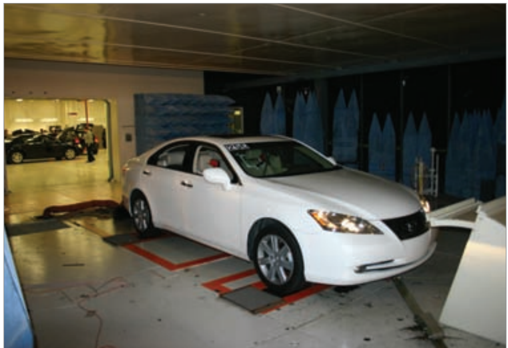
Figure 1: A vehicle positioned in a vehicle TEM cell
