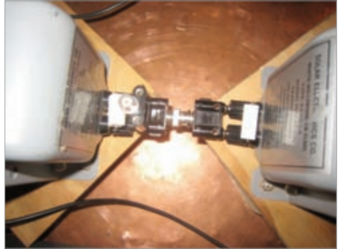
Figure 13: DM measurement connection close-up. The EMI receiver connection shown in Figure 10 is there, but the connecting coaxial cable has been removed for clarity.
