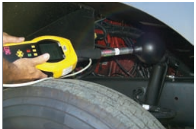
Figure 7: Example of magnetic field probe measurement
