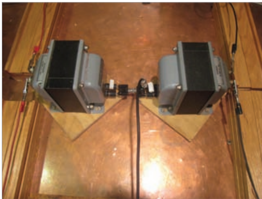
Figure 11: CM/DM measurements made using a pair of Solar 6220-1 coupling transformers. The connection of the primaries (expanded on in Figures 12 and 13) determines which mode is measured and which rejected.
