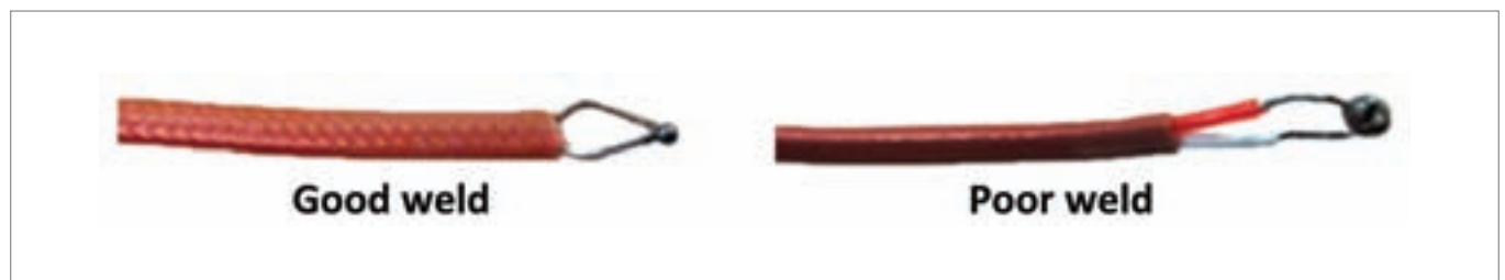
Figure 2: Good weld vs. poor weld
