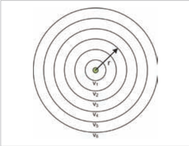
Figure 1: The fall-off of GPR with distance from the strike, where V_1 > V_2 > V_3 \dots etc.
