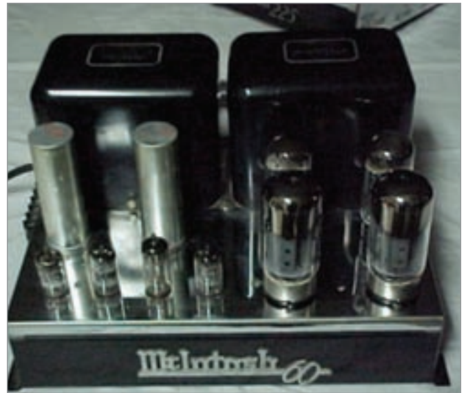
Figure 3: McIntosh MC60 amplifier specified for use with Solar 6541-1 in LSP-530-001
