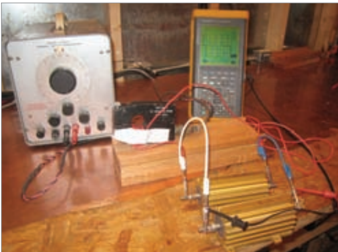
Figure 5: The 6541-1, center, with ten turns through the window is driven from the 100 watt Solar 6550-1 power audio oscillator and induces the oscilloscope-measured potential across the two parallel 1 ohm resistors in the foreground.
