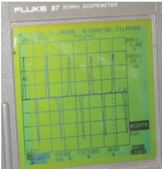
Figure 6a: 1 Vrms injected across 0.5 ohm at 30 Hz. Note considerable distortion, which can be ameliorated by more turns.
