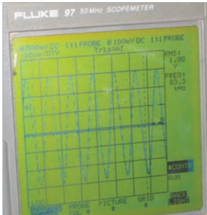
Figure 6c: 1 Vrms injected across 0.5 ohm at 80 kHz.
