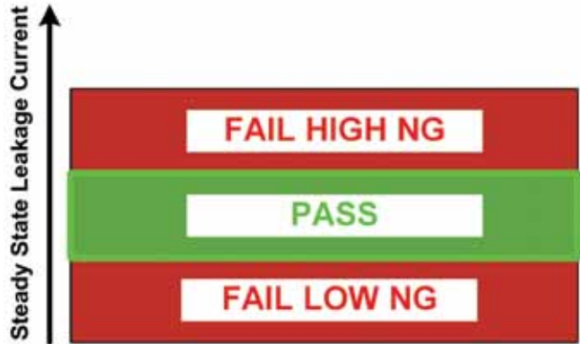
Figure 1: Pass Fail ranges for a hipot test
