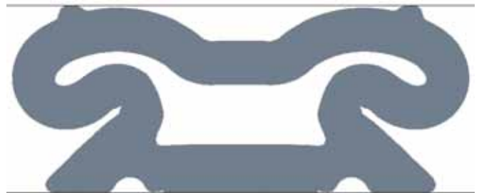
Figure 7: Single Gasket with Multiple Contact Points
